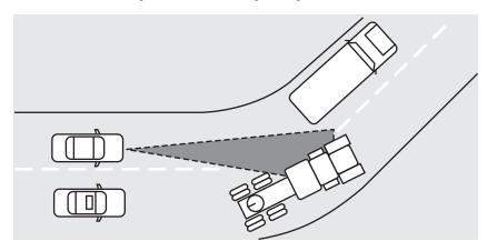
• There may be issues with the detection of vehicles in front when driving into and coming out of a bend or curve in the road.
